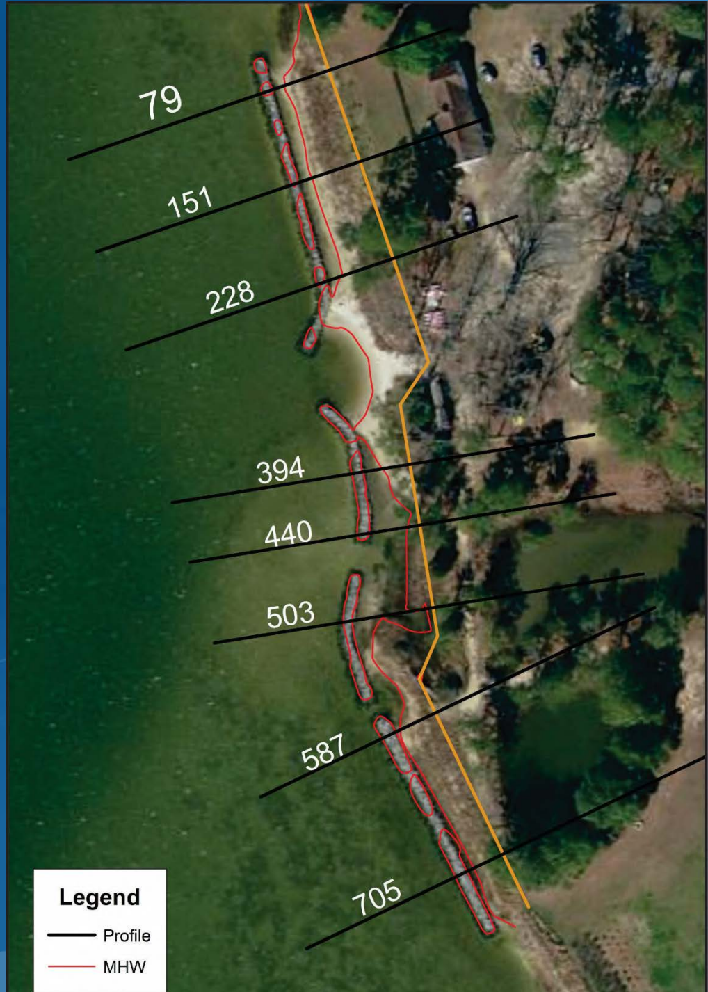
Location of cross-sectional profiles At Occohannock and the 2018 surveyed position of mean high water.
