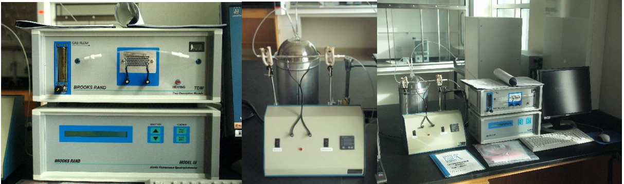
Brooks Rand thermal decomposition, GC separation, and atomic fluorescence instrumentation used for methylmercury measurement.
