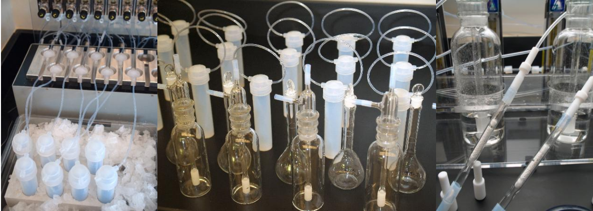
Extraction and ethylation equipment used to prepare water, sediment, soil, and biological samples for methylmercury analysis.
