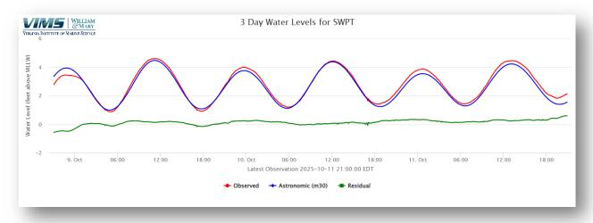
**Figure 1.** Example VIMS Tidewatch Chart of 3-Day hindcast data at NOAA's Sewells Point tide gauge, in Norfolk, VA, looking backward 72 hours since October 11, 2025 at 21:00 EDT (2025-10-12T01:00:00Z).
