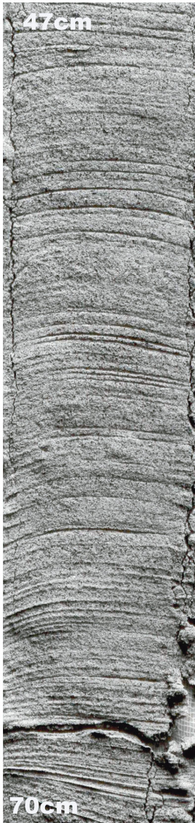
FIG. 12.—Lacquer peel from the sandy topset region showing thin lamination throughout.
