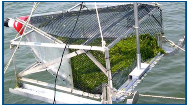
Seed Sled: This sled is used for collecting eelgrass seeds for use in restoration projects. Photo courtesy of Dr. Robert “JJ” Orth.
