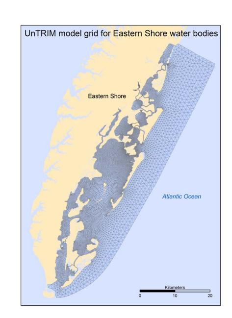
Figure 2. UnTRIM model grid for water bodies on ocean side of Eastern Shore.
