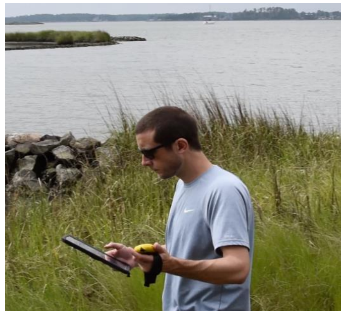
Fig 4. Use of a tablet and GPS survey tool connected via Bluetooth for increased accuracy.
