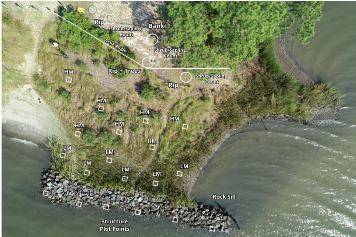
Fig 30. Detailed depiction of random plot locations for a monitoring site with one living shoreline treatment ( marsh with rock sill ).
