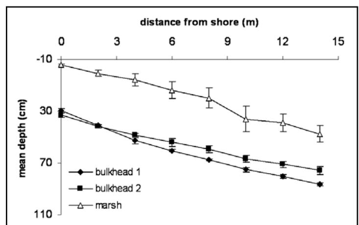
**Figure 1.** Water depth profiles at one fringe marsh and two bulkhead (BH) sites at Norman’s Creek. Means  $\pm$  SE are plotted ( $n=6$  for all data points). The College Creek site had a similar pattern, though depth at the bulkhead was deeper (60 cm).
