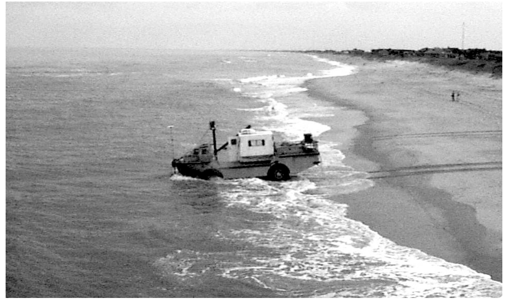
VIMS researcher Jesse McNinch is using a 5-ton amphibious vehicle to study erosional "hotspots." The vehicle can reach speeds of 5 knots in the water and operate up to 5 miles offshore.
