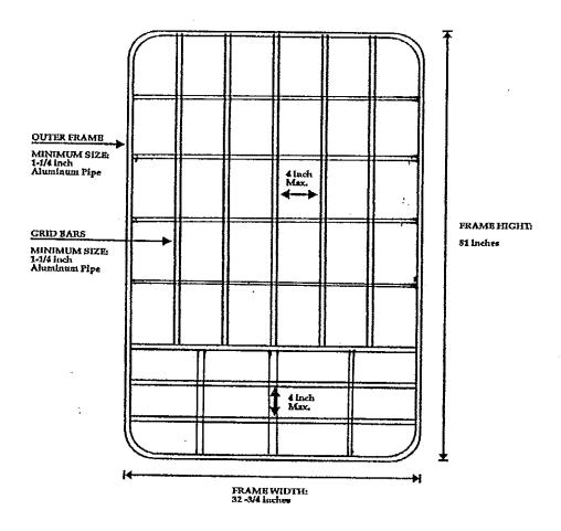
The modifications were welded aluminum round stock, the same as the TED's construction, with the goal of providing fish an avenue of escape, while being strong enough to withstand the chafing of scallops going through. This shooter was installed as a TED would be, with an escape hole at the top, except without the covering flap and at a slightly greater angle, 35-40% vs 45%.
