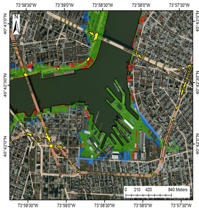
Figure 9. Area comparison results after underpass inclusion, with highway underpasses shown in yellow for Brooklyn near the Navy Yard. Of the 66 underpasses shown, 15 (22.7%) are within the storm surge impact area of Hurricane Sandy.
