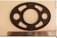
Figure 1. PHA biodegradable escape panel for blue crab traps.
