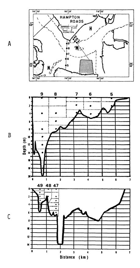
Figure IIA-14. Current measurement stations near Newport News Point occupied during "Operation James River-1964". A: Station locations, Mouth of Nansemond River (N) Hampton Flats (H) and Newport News Middle Ground Shoal (M) are identified; B: Measurement depths south of Newport News Point; C: Measurement depths across Newport News Bar. Dotted polygons in B and C delineate portions of cross-sectional area applied to currents to obtain instantaneous transport.
