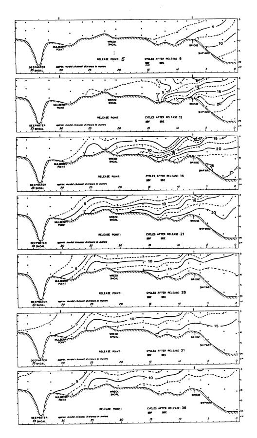
Figure IIA-9a SBF dye concentrations (ppb) along the axis of the James resulting from injection near the mouth of the Nansemond River (5 in Figure IIA-5).
