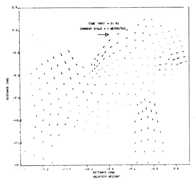
Figure IIIE-14c. Flow field in Hampton Roads, Island D, slack before flood.
