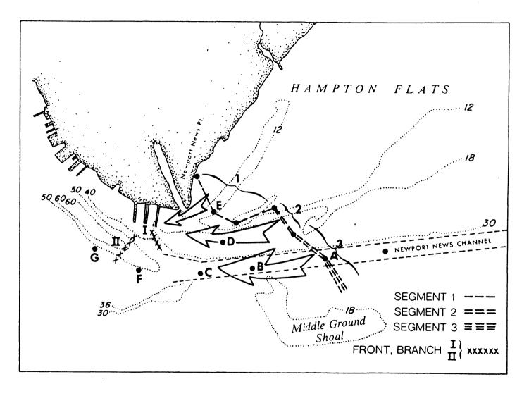
Figure IVA-2a. Segments used in calculation of flux to the frontal system, BASE condition. Reference text for details.
