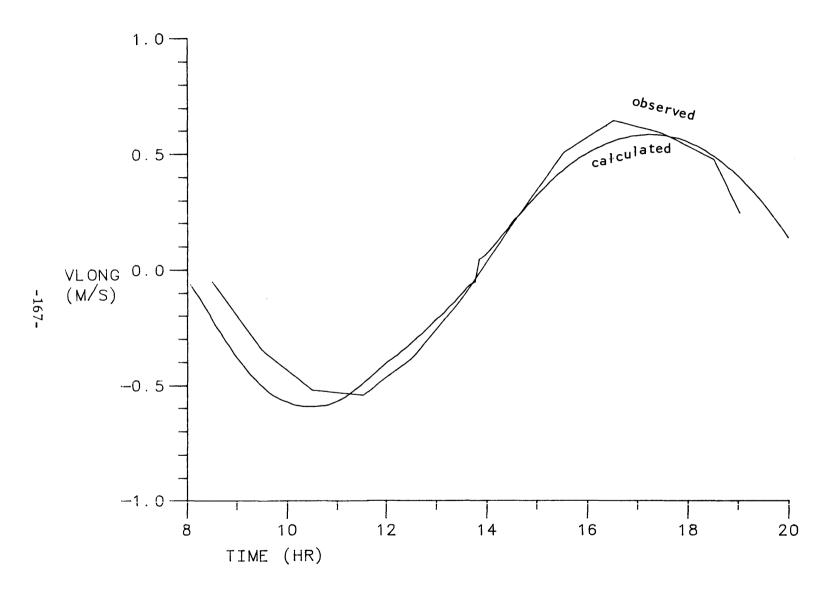
Figure IIIE-8 Comparison of Observed Current at Station H13 with Model Prediction
