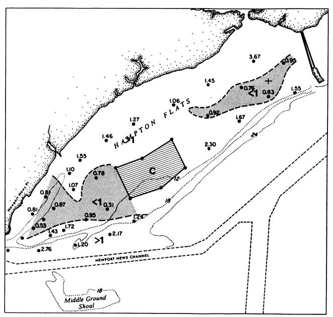
Figure IIIF-12a. Values of  $\tau_{\text{O}}/\tau_{\text{C}}$  for Island C, maximum flood current.
