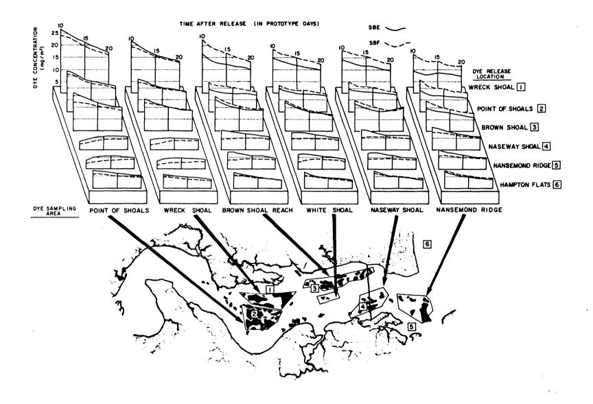
Figure IIA-6. Lower portion: Dye injection locations and oyster rock regions of interest.
