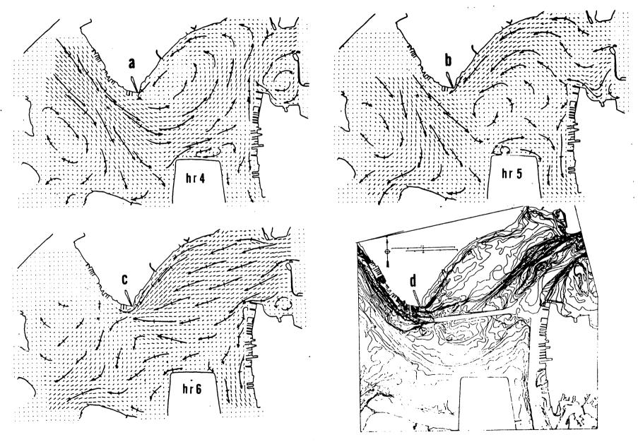
Figure IIA-13. Surface circulation in the James River Hydraulic model (Hampton Roads portion) at lunar hour 4 (a), 5(b) and 6(c) and bathymetry of Hampton Roads (d) at 2 ft intervals.
