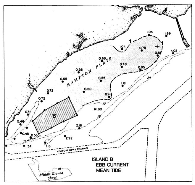
Figure IIIF-11b. Values of  $\tau_{\text{O}}/\tau_{\text{C}}$  for Island B, maximum ebb current.
