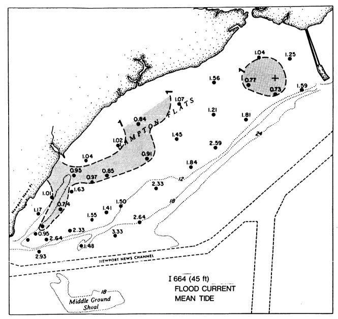
Figure IIIF-8a. Values of  $\tau_0/\tau_C$  for 1664 (45 ft), maximum flood current.
