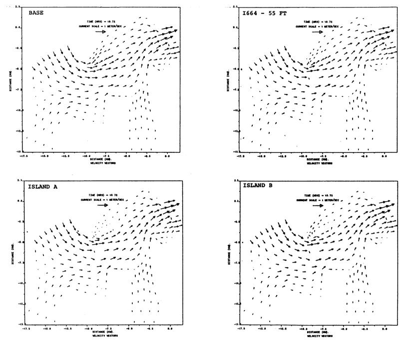
Figure IIIE-12b. Flow field in Hampton Roads, maximum ebb.
