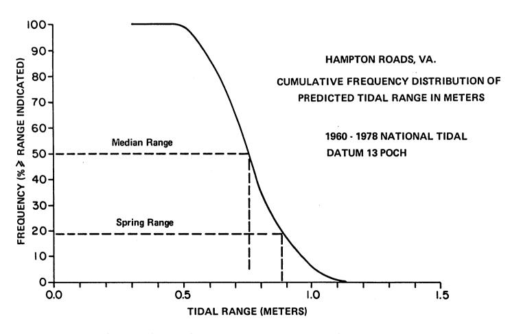
Figure IIIF-5. Cumulative distribution of tide range for 1960-1978 Tidal Datum Epoch.
