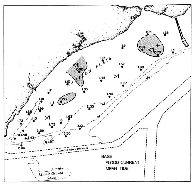
Figure IIIF-4a. Values of  $\tau o/\tau_C$  for BASE condition, maximum flood current.
