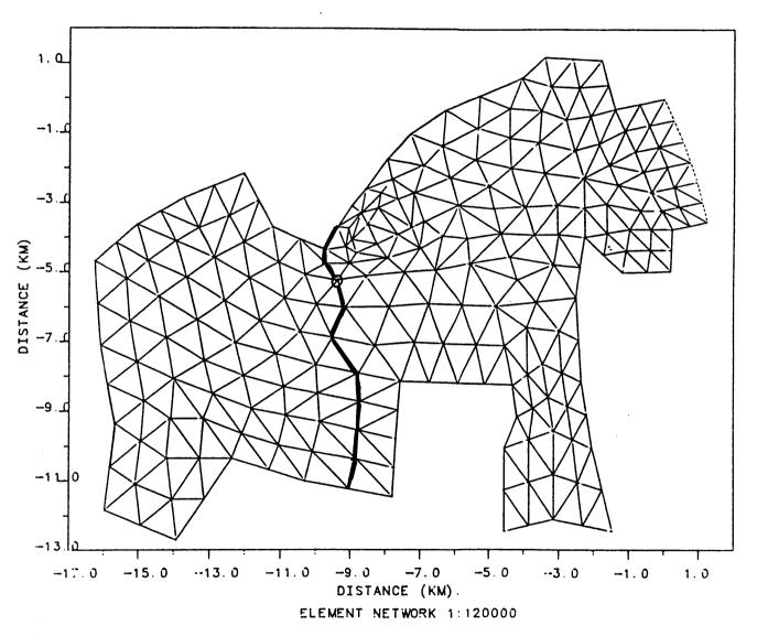
Figure IIIE-9. North-South transect for flux calculations shown in Table IIIE-3. Circle represents Node 125, South Island of 1664.
