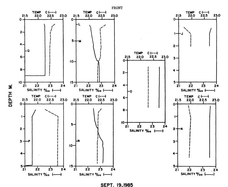
Figure IIIB-3. Temperature and salinity profiles for water column stations J-Q inclusive, as sampled on Sept. 19, 1985. Depth of sampling indicated by corresponding letter on the figure. The surface frontal feature is between samples L-N (west of front) and O (east of front). For sample location see Figure IIIB-1.
