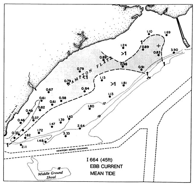
Figure IIIF-8b. Values of  $\tau_{0}/\tau_{C}$  for I664 (45 ft), maximum ebb current.
