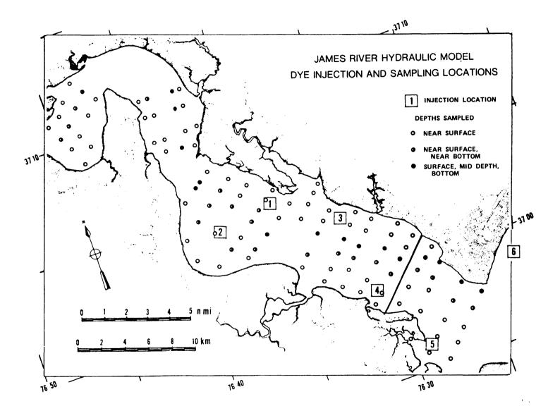
Figure IIA-5. Dye injection and sampling locations in a portion of the James River Hydraulic model. (After Ruzecki and Hargis, 1985).
