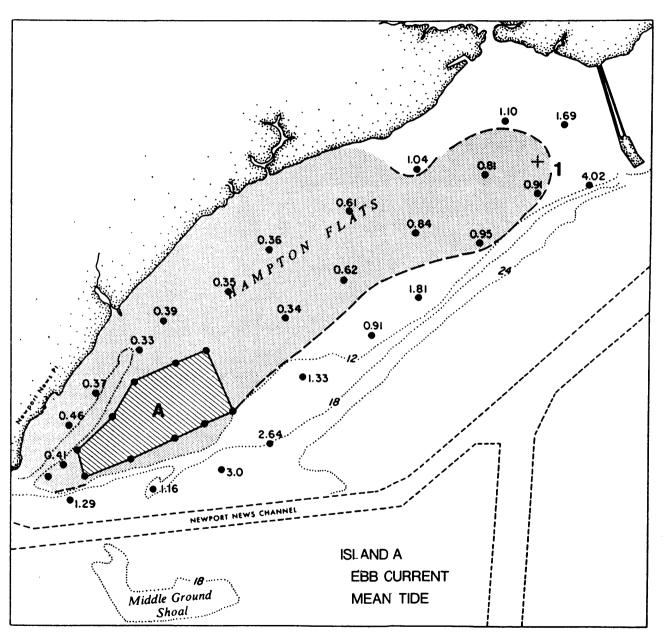
Figure IIIF-10b. Values of  $\tau_{\text{O}}/\tau_{\text{C}}$  for Island A, maximum ebb current.
