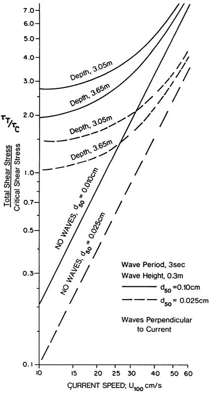
Figure IIIF-6 Total bottom shear stress to critical shear stress due to wave-current interaction.
