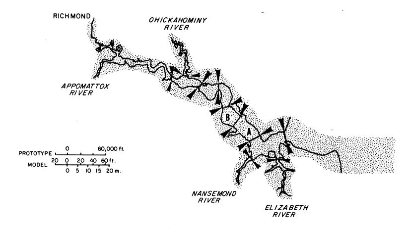
Figure IIA-19 James River Hydraulic Model segmentation with dams after dye experiments.
