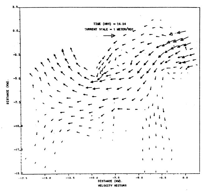
Figure IIIE-14a. Flow field in Hampton Roads, Island D, maximum flood.
