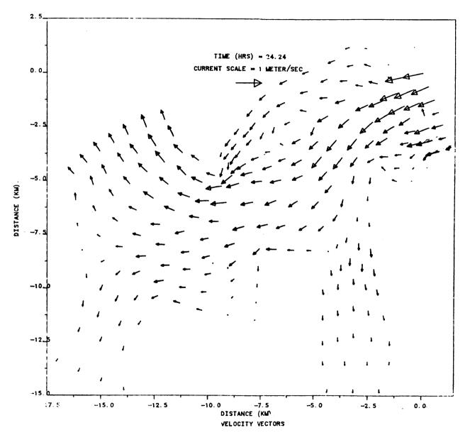
Figure IIIE-13a. Flow field in Hampton Roads, Island C, maximum flood.
