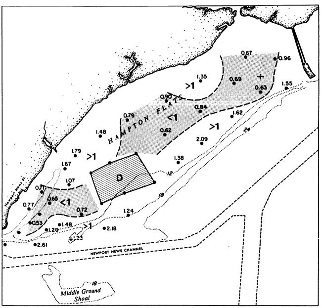
Figure IIIF-13a. Values of  $\tau_0/\tau_c$  for Island D, maximum flood current.
