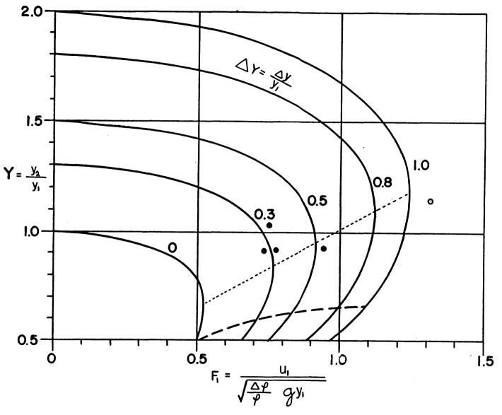
Figure IIID-2. Front characteristics as dimensionless function of the densimetric Froude number, with demensionless bottom change  $\Delta Y$  as parameter. (The experimental data point o is for  $\Delta Y$  = 1.0 data point • is for Y = 0.3)
