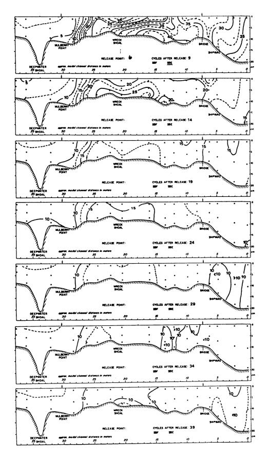
Figure IIA-8b SBE dye concentrations (ppb) along the axis of the James resulting from injection at Hampton Flats (6 in Figure IIA-5).
