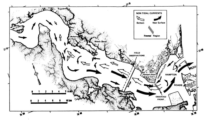
Figure IIA-10. Hypothesized surface and bottom non-tidal circulation in the James River Estuary based on variations in dye concentrations (after Ruzecki and Hargis, 1985).
