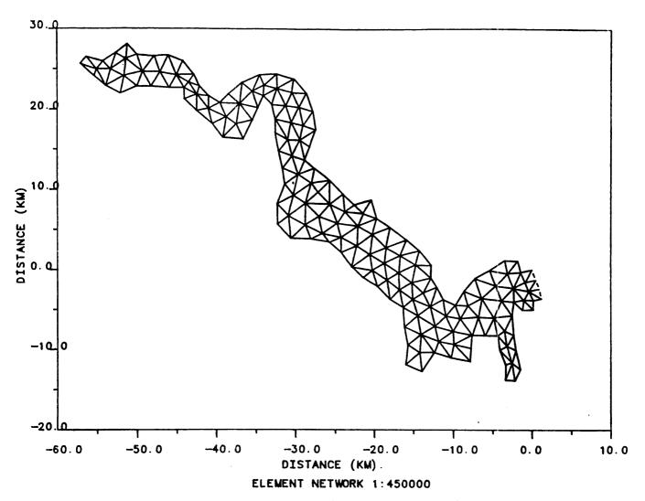
Figure IIIE-1 Large-scale two dimensional model grid for James River
