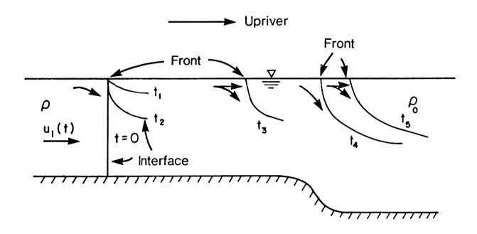
Figure IIID-3. Conceptualized model of front evolution along the Newport News Channel.
