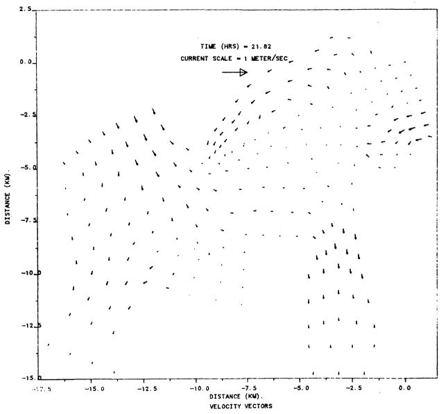
Figure IIIE-13c. Flow field in Hampton Roads, Island C, slack before flood.
