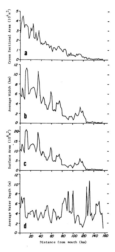
Figure IIA-3. Variations in geometry of the James River Estuary as a function of distance upstream: a)Cross sectional area; b)Average width; c)Surface area; and d)Average cross sectional depth.
