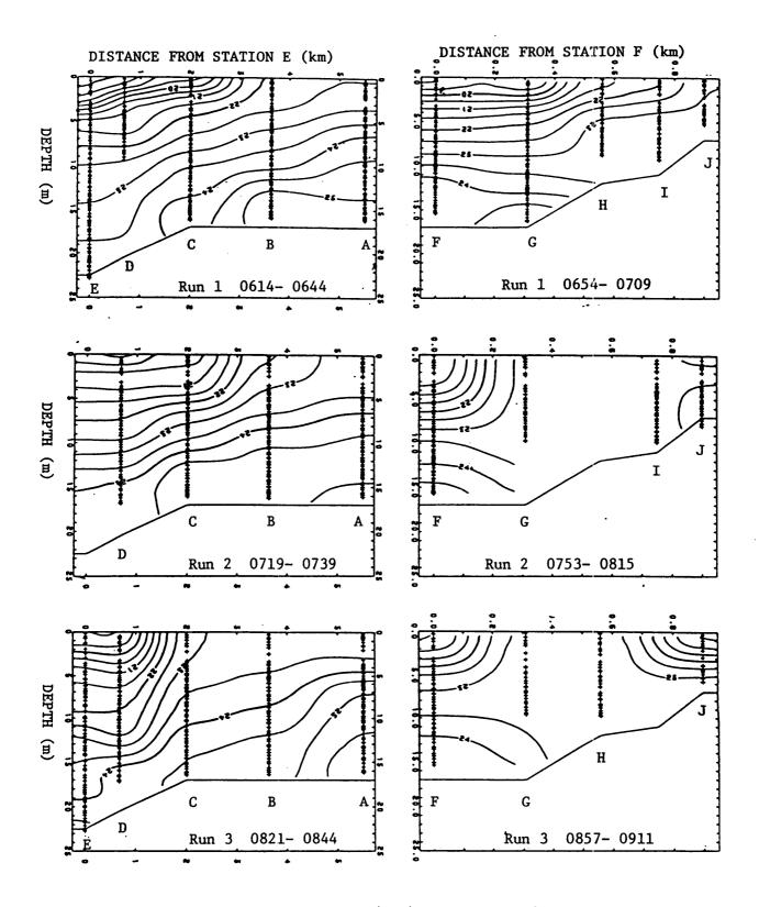
Figure IIIA-5. Salinity distribution (ppt), June 19, 1985 along transects shown in Figure IIIA-4. The "+" symbols indicate the location of each data point.
