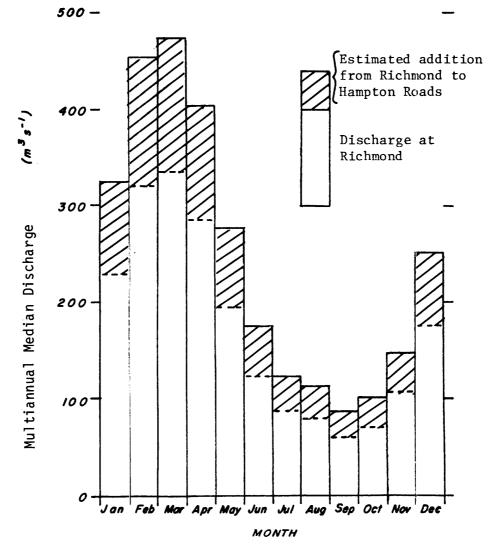
Figure IIA-4. Estimated monthly median discharge of fresh water into the James River based on records from 1925 to 1975 taken at Cartersville, Va. and corrected to include total drainage basin (to Hampton Roads).
