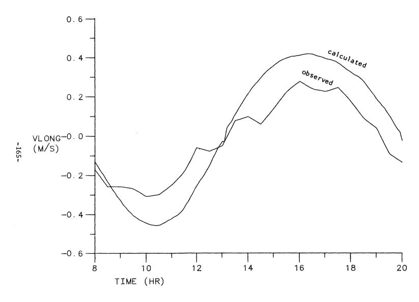
Figure IIIE-7 Comparison of Model Prediction with Observed Current at Station C3
