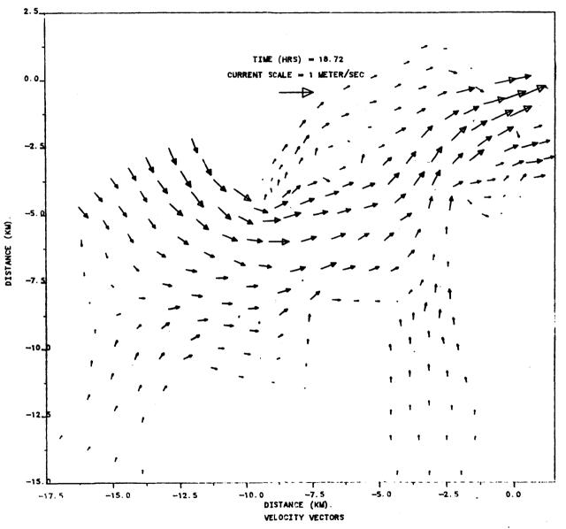
Figure IIIE-14b. Flow field in Hampton Roads, Island D, maximum ebb.
