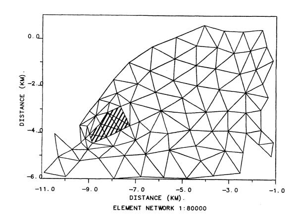
Figure IIIE-3 Model Grid Configuration for Island A
