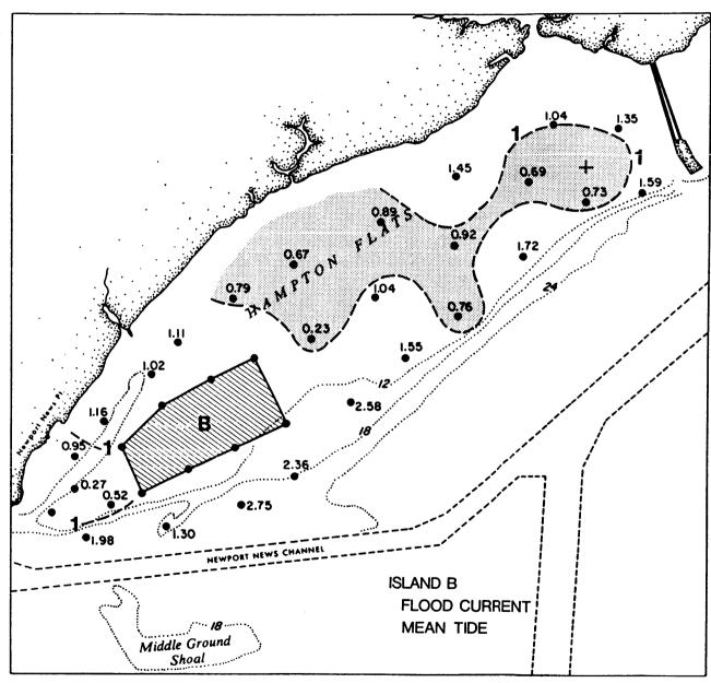
Figure IIIF-11a. Values of  $\tau_{\text{O}}/\tau_{\text{C}}$  for Island B, maximum flood current.
