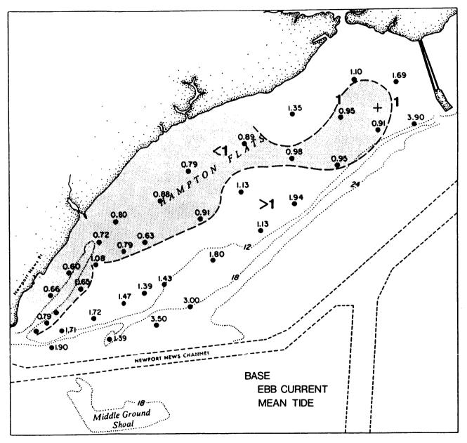
Figure IIIF-4b. Values of  $\tau_{\text{O}}/\tau_{\text{C}}$  for BASE condition, maximum ebb current.
