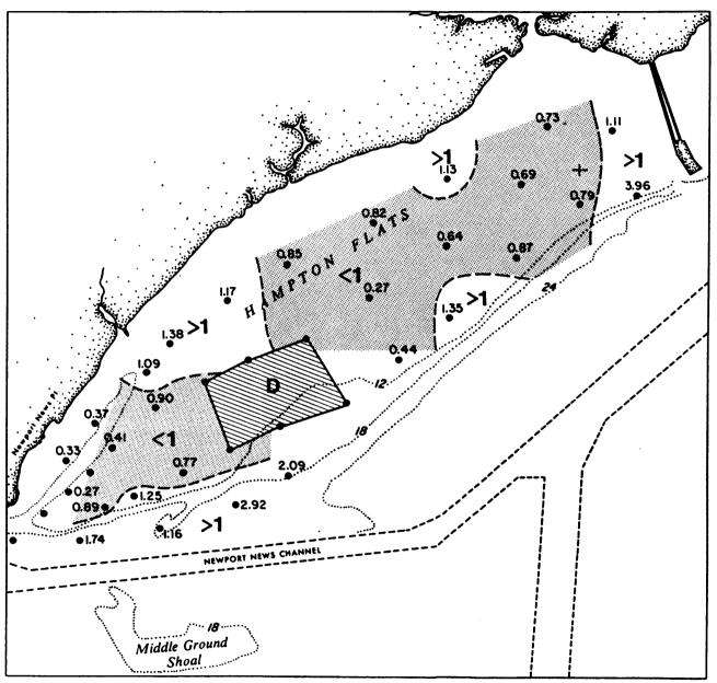
Figure IIIF-13b. Values of  $\tau_{\text{O}}/\tau_{\text{C}}$  for Island D, maximum ebb current.
