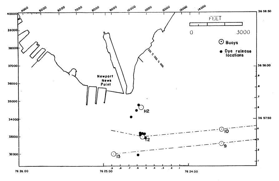
Figure IIIA-2. Locations of dye release to trace the path of surface water across the frontal system.
