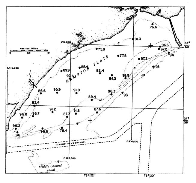
Figure IIIF-2. Percent weight of sand fraction.
