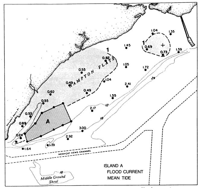
Figure IIIF-10a. Values of  $\tau o/\tau_C$  for Island A, maximum flood current.
