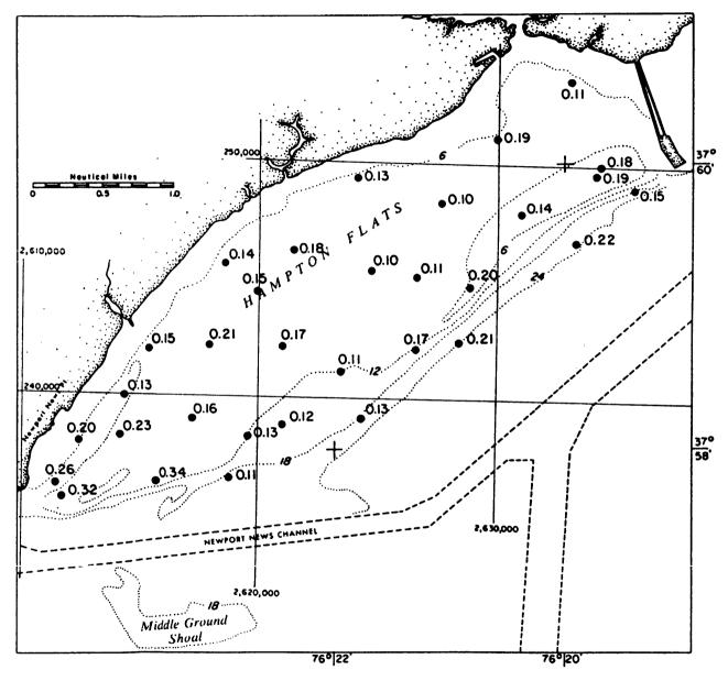
Figure IIIF-1. Median grain size of sand fraction, mm.
