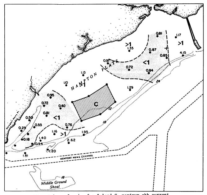
Figure IIIF-12b. Values of  $\tau_{\text{O}}/\tau_{\text{C}}$  for Island C, maximum ebb current.
