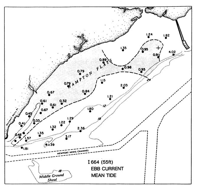
Figure IIIF-9b. Values of  $\tau_{\text{O}}/\tau_{\text{C}}$  for I664 (55 ft), maximum ebb current.
