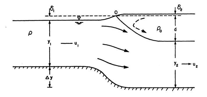
Figure IIID-1. Definition sketch for the analysis of diving of heavier fluid at front.
