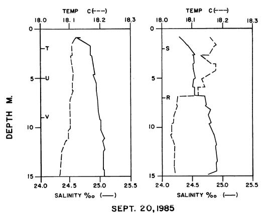
Figure IIIB-4. Temperature and salinity profiles for water column at stations R-V inclusive, as sampled on Sept. 20, 1985. Depth of sampling indicated by corresponding letter on the figure. For sample location see Figure IIIB-1. The position of the surface frontal feature lies between samples T-V inclusive (to west of front), and S-R inclusive (east of front).
