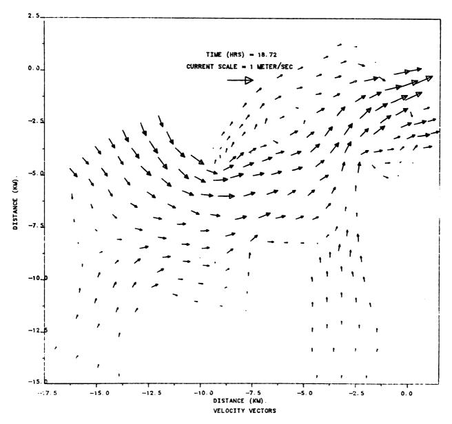
Figure IIIE-13b. Flow field in Hampton Roads, Island C, Maximum ebb.
