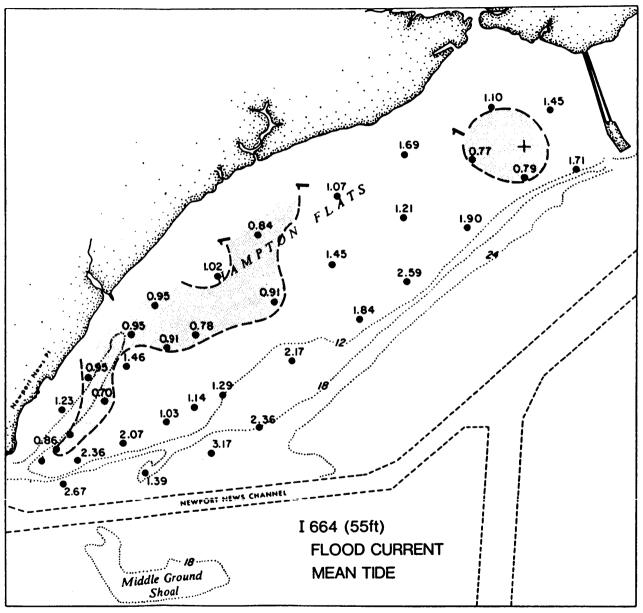
Figure IIIF-9a. Values of  $\tau_0/\tau_C$  for 1664 (55 ft), maximum flood current.
