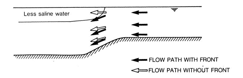
Figure IVA-1. Effect of front on flow displacement.
