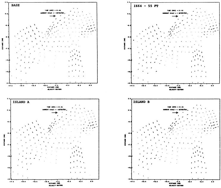
Figure IIIE-12c. Flow field in Hampton Roads, slack before flood.
